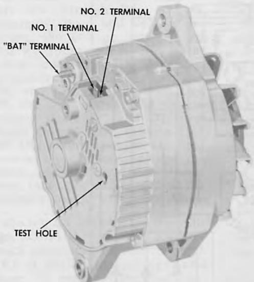
Figure 3—Typical 27-SI Series generator.
