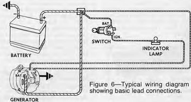
Figure 6—Typical wiring diagram showing basic lead connections.
