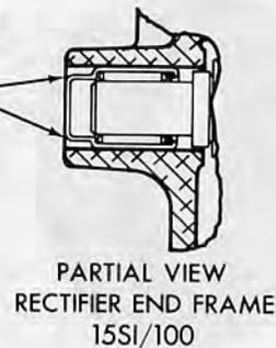
Figure 17—Slip ring end frame bearing assembly, 15-SI.
