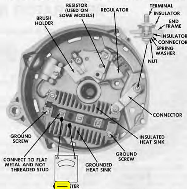
Figure 11—Rectifier bridge check, 10-SI
