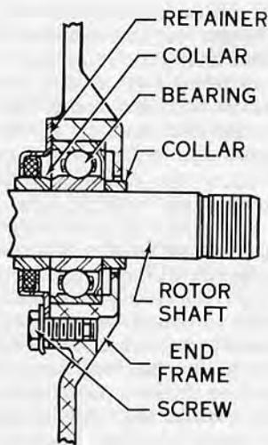
Figure 16—Drive end bearing assembly, 15-SI.
