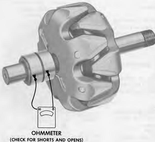
Figure 8—Checking rotor winding.
