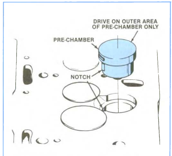
Figure 3-7, Pre-Chamber Installation in Cylinder Head.
