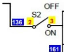
For example **136** shows base number wire 136 is connected to S2-2 and base wire number 161 is connected to S2-3.
