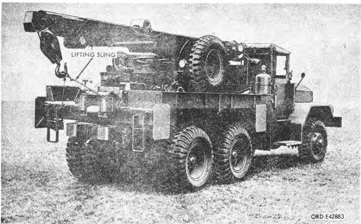
Figure 55. Securing crane for traveling.
