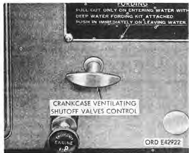
Figure 79. Crankcase ventilating shutoff valves control.
