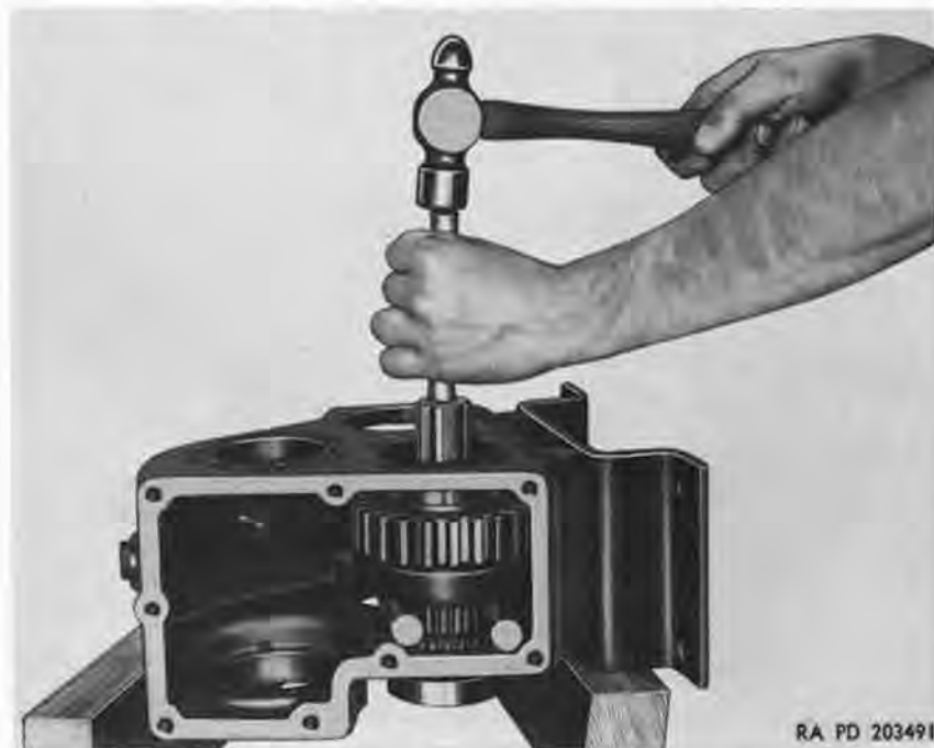
Figure 92. Removing input shaft.
