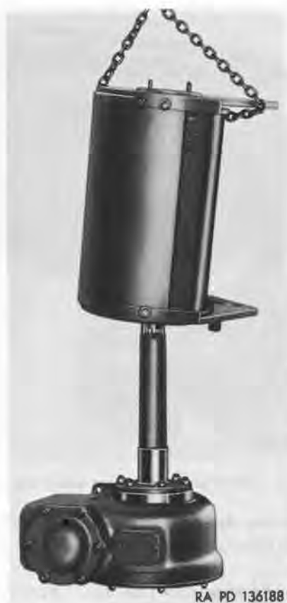
Figure 36. Separating hoist drum from worm and drive gear set.
