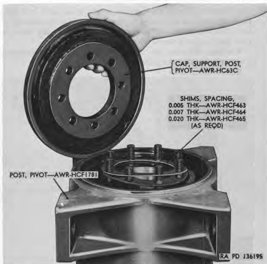
Figure 43. Removing pivot post support cap and spacing shims.
