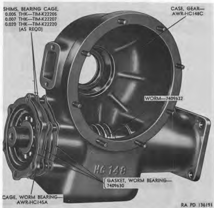
Figure 39. Worm partially removed from gear case.
