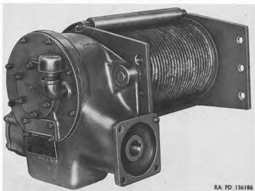
Figure 34. Hoist drum and worm and drive gear set.
