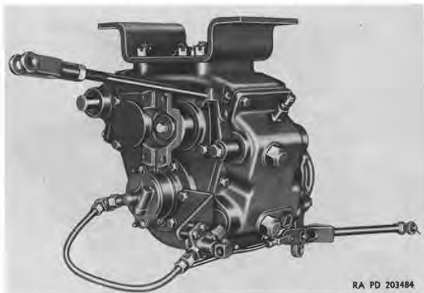
Figure 85. Power divider with levers and governor assembly attached—left front view.
