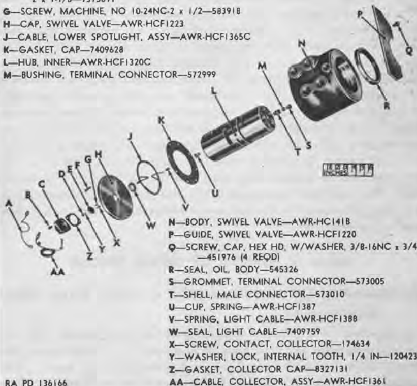
Figure 14. Swivel valve assembly—exploded view.
