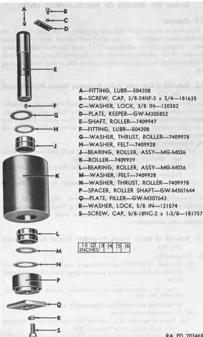
Figure 70. Vertical cable guide roller—exploded view.
