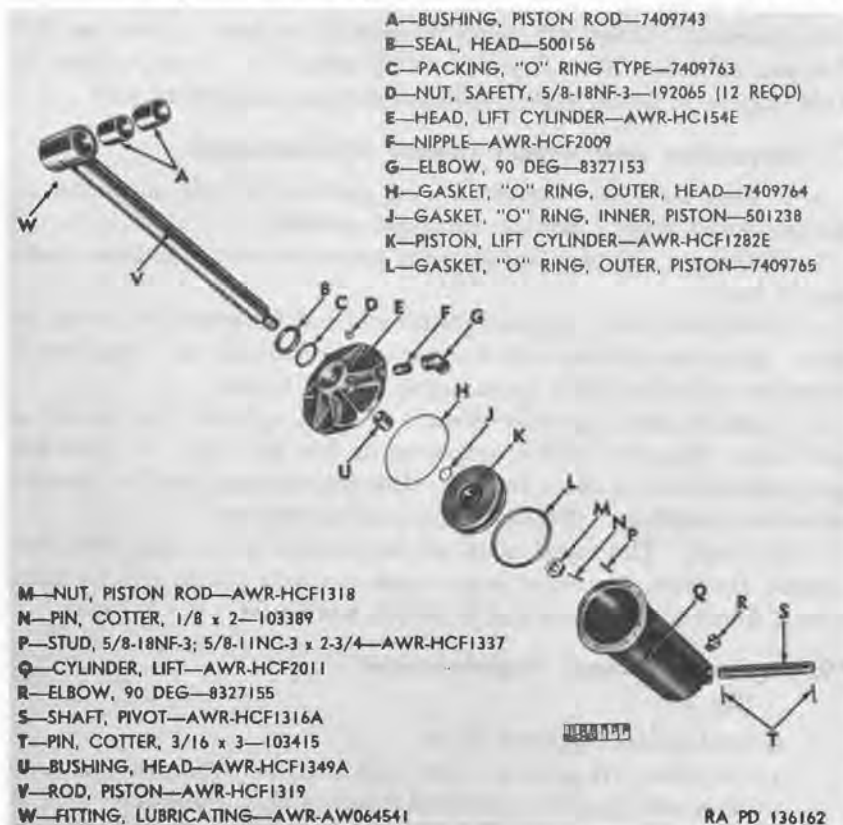
Figure 10. Lift cylinder—exploded view.
