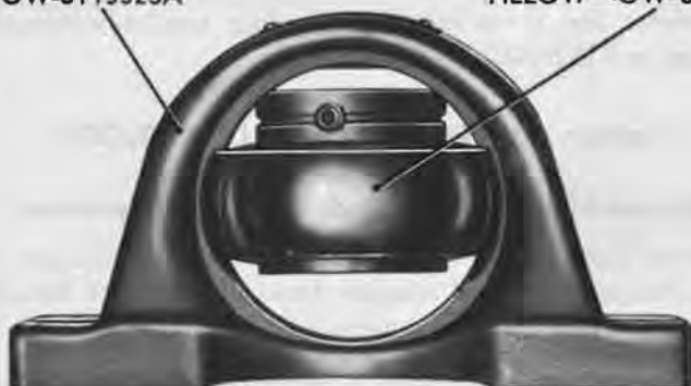
Figure 101. Positioning pillow block bearing for removal.
