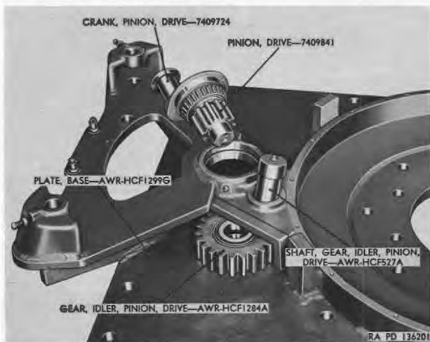
Figure 49. Pivot post drive pinion and drive pinion idler gear removed
