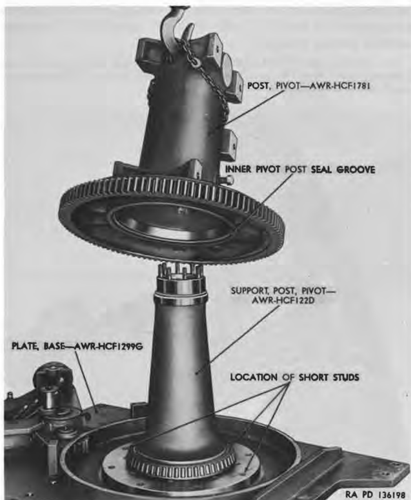
Figure 46. Removing pivot post from base plate.
